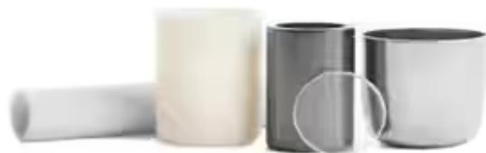
The Crystal Polishing Kit contains everything needed by the spectroscopist for repolishing and buffing most infrared transmission crystals, including KRS-5. Two ground glass discs are provided /n--one for fine grinding and the other to which self-stick polishing pads may be affixed.
