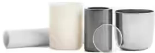
The POCO graphite electron beam evaporation crucibles are designed to offer E-Beam users improved evaporation performance over that obtainable in bare hearth mode. Our graphite crucible acts as an energy efficient thermal barrier between the molten evaporant and the water cooled copper hearth.
