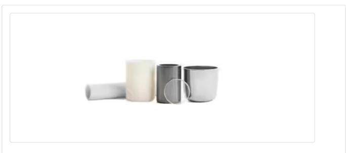
In the analytical laboratory, nickel crucibles offer high resistance to dilute alkalies at a very low cost per crucible. In some instances, nickel crucibles are preferable to zirconium: for instance, sodium peroxide fusions in which zirconium itself is to be determined; also in analysis for columbium (niobium), tantalum or low phosphorus.
